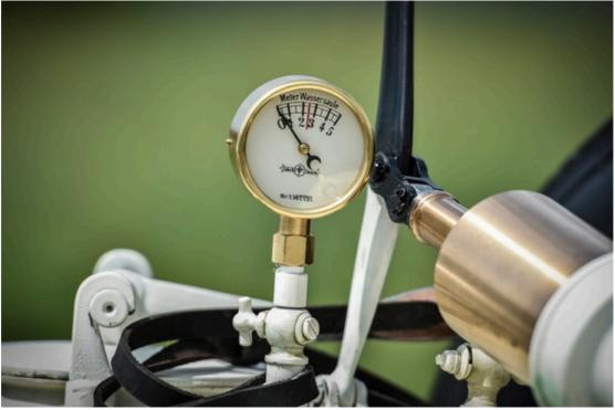
Glance right and there's an angled pressure gauge fronting a village pump. To maintain fuel flow it's your job to watch the gauge. Should its needle flick left below 1Kg/sq.cm. you tug at the pump handle like an exasperated Dutchman at a
