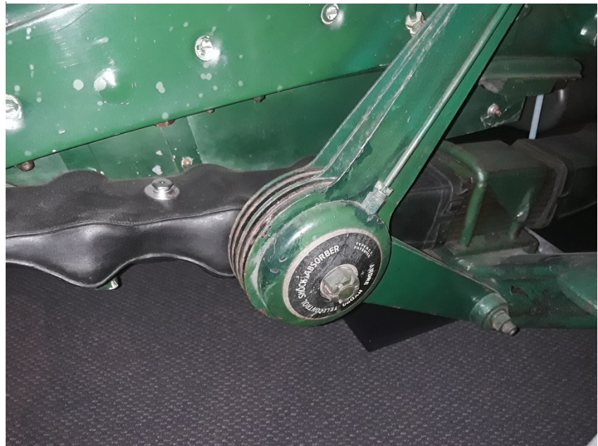
Friction Dampers (or shock absorbers) - Eric Jensen Photo
