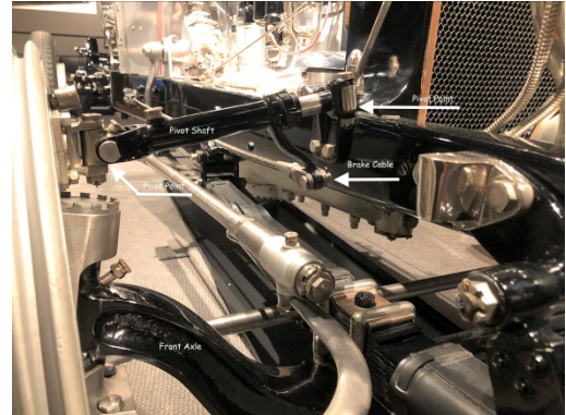
Hispano-Suiza Chassis Front Brake System
