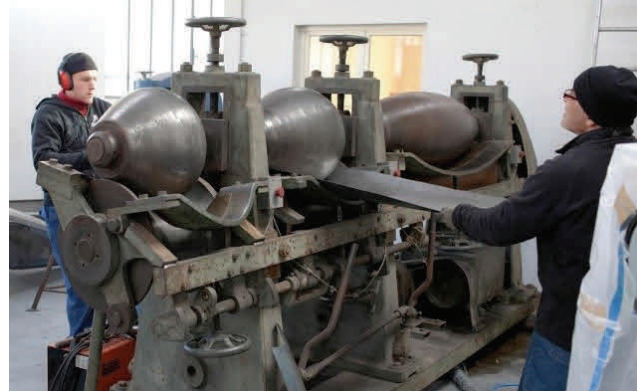
Three Olive Machine powered by an electric motor
