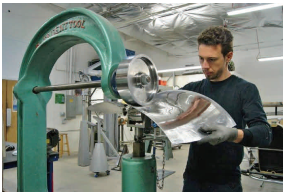
The English wheel used for smaller panels
